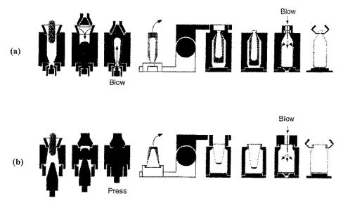
**Fig. 9.10** Methods of forming glass containers: (a) blow and blow forming, (b) press and blow forming for wide-mouthed containers; by courtesy of Rockware Glass Ltd.
