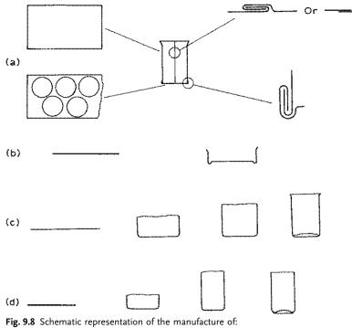
(a) three-piece can, (b) drawn can, (c) drawn and redrawn can, (d) drawn and wall-ironed can; from [15] with permission of the authors.
