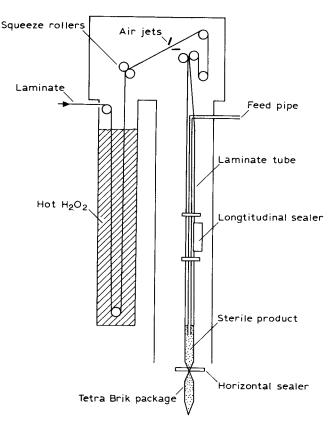
Fig. 9.13 Principle of the Tetra Brik aseptic packaging system; from [15] with permission.
