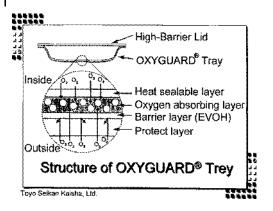
**Fig. 9.14** Structure of the Oxyguard tray.
