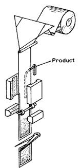
**Fig. 9.1** Vertical form-fill-seal machine for sachets; adapted from [16] with permission.
