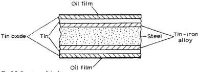
Fig. 9.5 Structure of tinplate.
