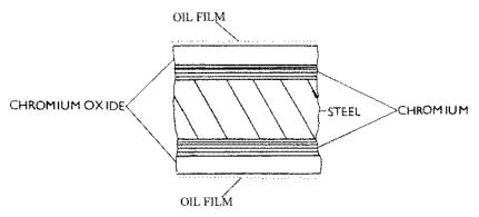
Fig. 9.7 Structure of ECCS plate (tin-free steel).
