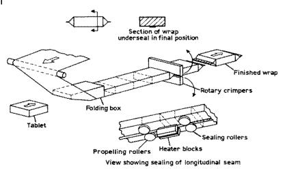
**Fig. 9.4** Horizontal form-fill-seal machine for pillow packs. Film is drawn from reel and formed into horizontal tube around product with continuous seal underneath formed by heater blocks and crimping rollers. Then, rotary heaters make the crimped end seals and cut-off produces individual packs. Adapted from [16] with permission.
